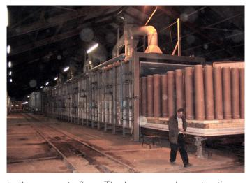
to the concrete floor. The burners and combustion control included 39 off TJ75 Thermjet medium velocity burners fired positioned three in each firing dike disposed as two burners from one side and one from the opposite side, incorporated in a 3 zone control.
